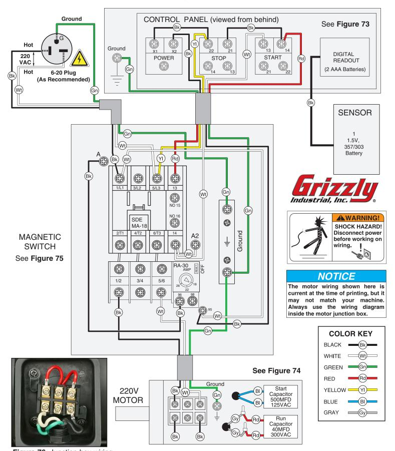
**Figure 76**. Junction box wiring.
